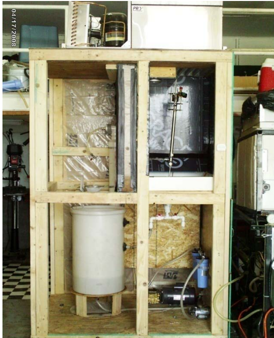
Figure 12. Batch Reactor System (Front View)
