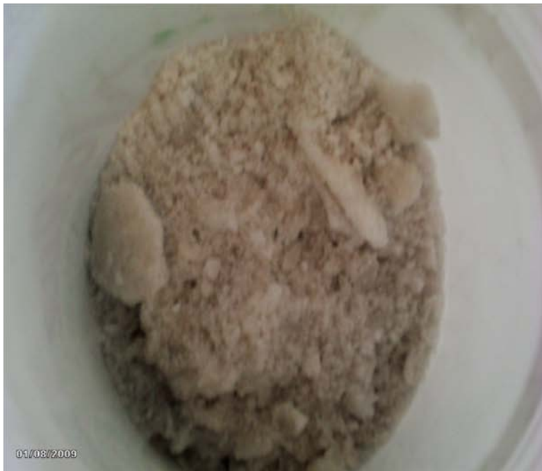
Figure 23. Hydrate Produced in the Bench-scale Batch Hydrate Reactor System
